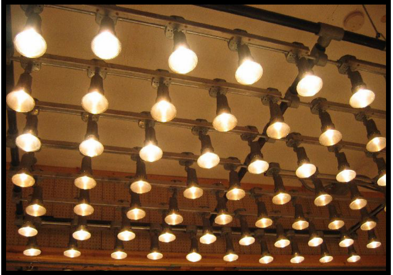
Figure 2. Lights generating the radiant load.
