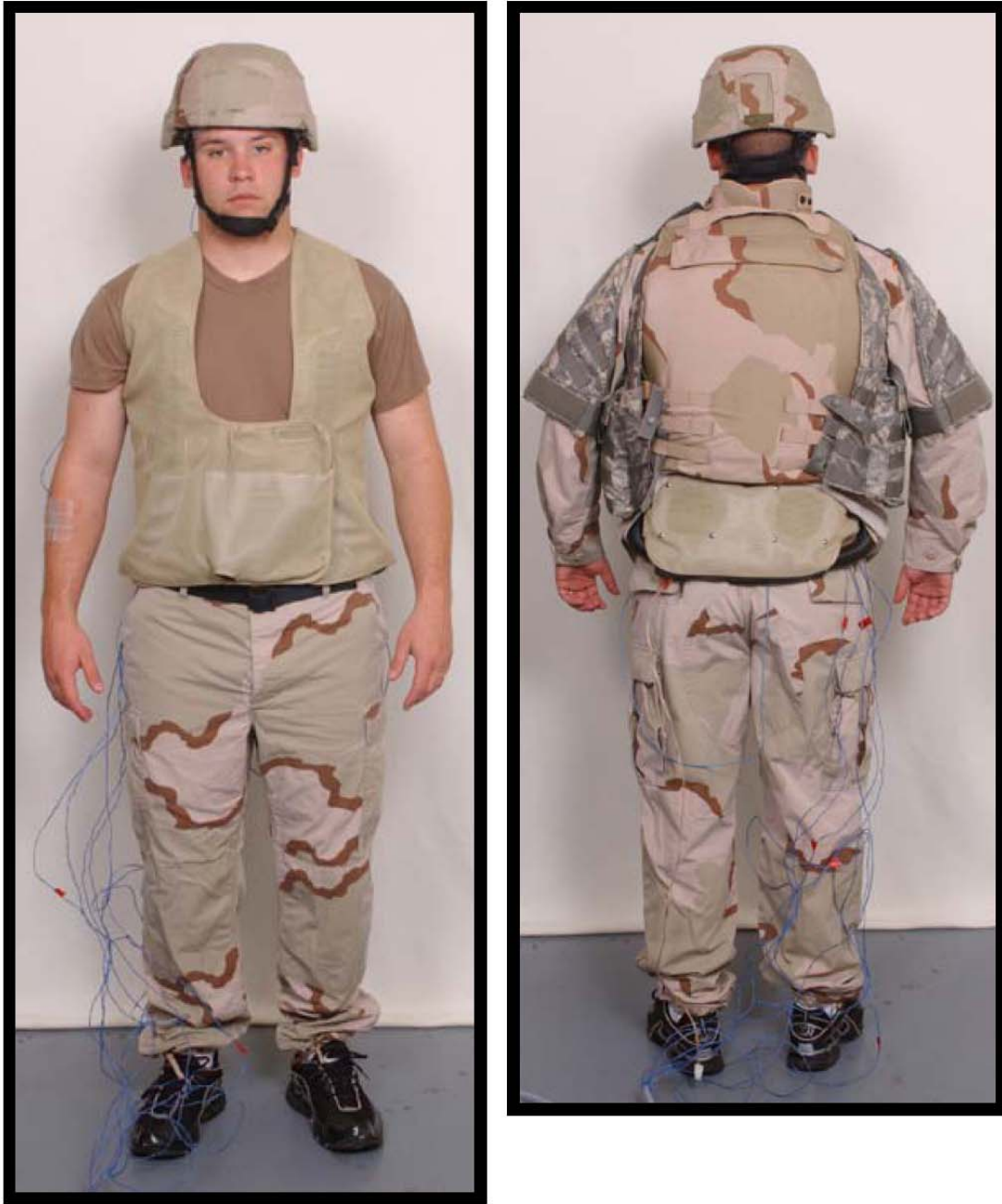
Figure 1-11. Subject dressed in PCS #10: Summitstone ForcedAir Vest (FAV3) worn over T-shirt and under DCU shirt.
