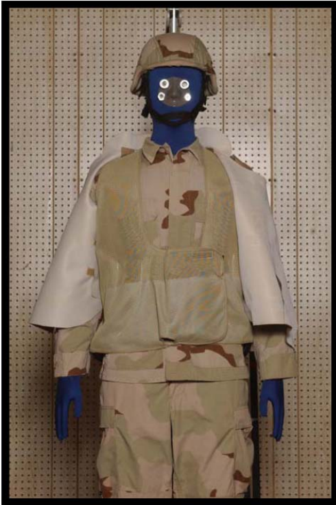
Figure 3. PCS #1: ClimaTech Safety ForcedAIR Vest 1 worn over the DCU shirt; vinyl vest is opened in left view and not shown in right view.
