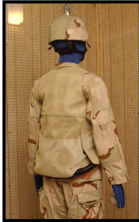
Figure 3. PCS #1: ClimaTech Safety ForcedAIR Vest 1 worn over the DCU shirt; vinyl vest is opened in left view and not shown in right view.
