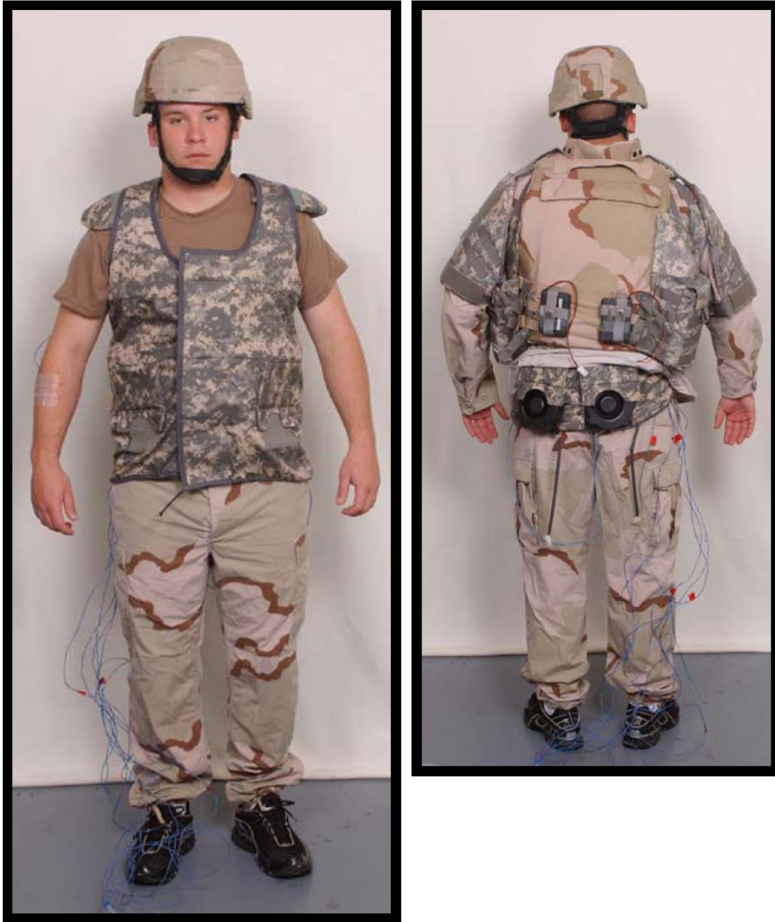
Figure 1-10. Subject dressed in PCS #9: Summitstone ForcedAir Vest – Redesigned (FAV2) and worn over T-shirt and under DCU shirt.
