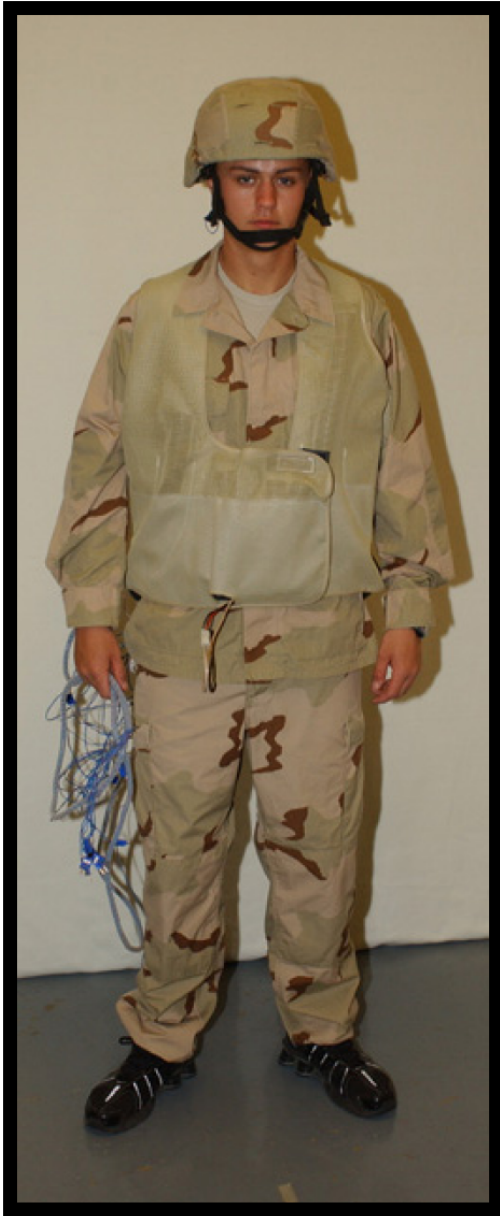
Figure 1-2. Subject dressed in PCS #1: Summitstone ForcedAir Vest (FAV1) worn over DCU shirt
